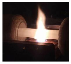
of approximately 0.020 or NA=0.25 with respect to pure silica. Above mentioned characteristics make OPD an ideal technology for production of triple-clad laser fiber preforms or custom-made silica-silica fiber preforms.
